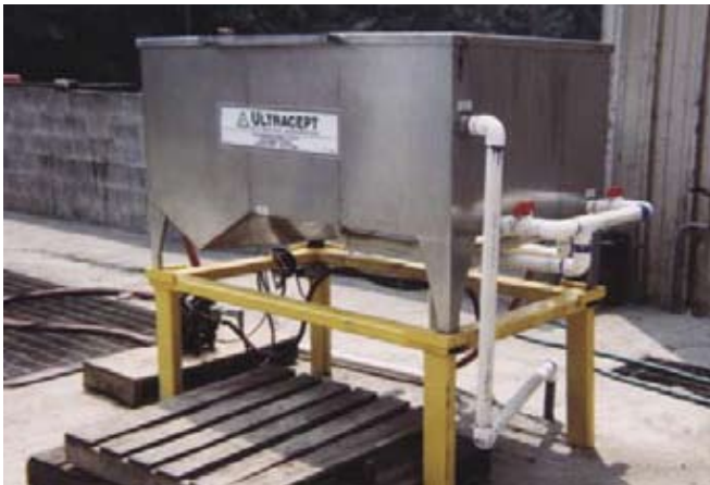
The Ultracept® Oil-Water Separator – Equipment Rental House, College Station, Texas
